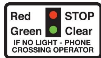
Miniature warning lights at level crossings
