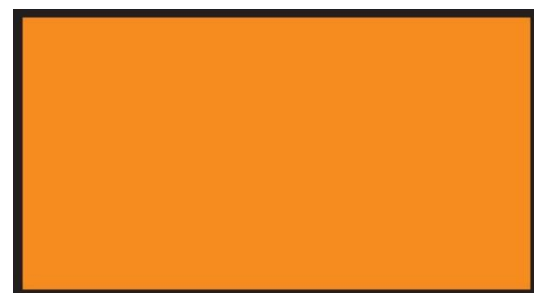
The above panel will be displayed by vehicles carrying certain dangerous goods in packages
