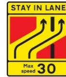
One lane crossover at contraflow road works
