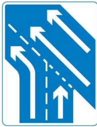
Traffic on the main carriageway coming from right has priority over joining traffic
