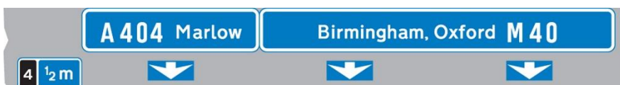
Downward pointing arrows mean 'Get in lane' The left-hand lane leads to a different destination from the other lanes.
