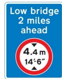
Advance warning of restriction or prohibition ahead
