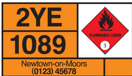
The panel illustrated is for flammable liquid. Diamond symbols indicating other risks include:
