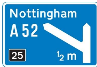
On approaches to junctions (junction number on black background)
